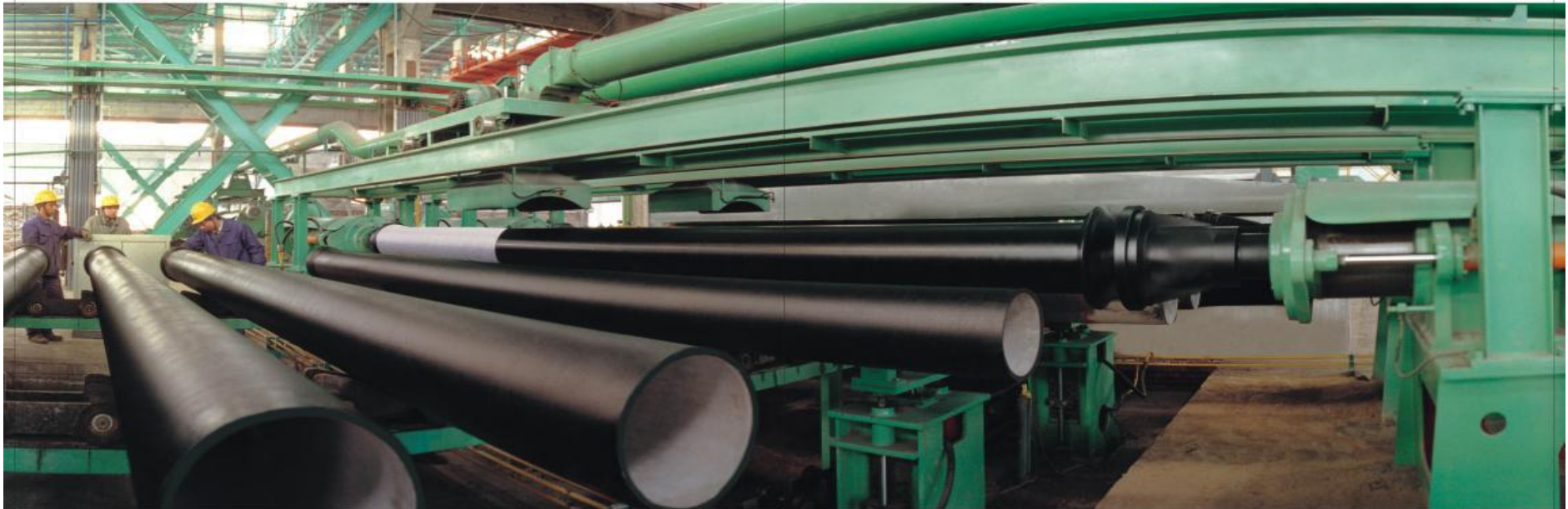
沥青喷涂 Bitumen coating
