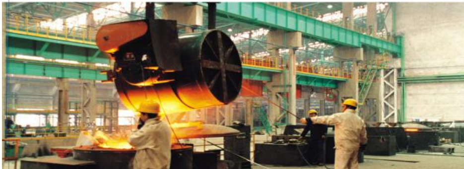
电炉升温及调质 Heating and spheroidization in induction furnace
