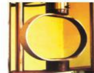
压环试验 Hardness test
