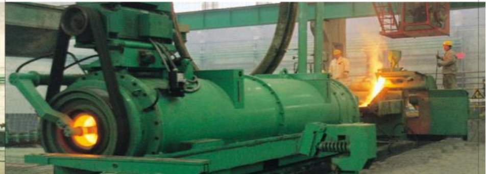
离心浇铸 Centrifugal casting
